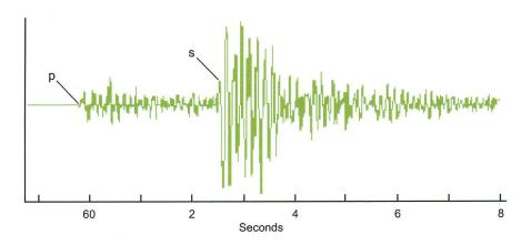
These signals are recorded with a very accurate time scale. Note the points labelled 'P' and 'S' on the signal. By measuring the time difference between these two points, and performing some calculations, it is possible to determine the distance from the sensor to the earthquake epicentre.
